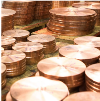
SEAM WELD WHEEL BLANKS
